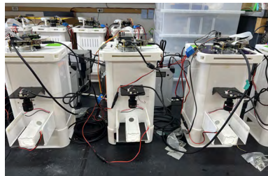
The BumbleBox is an automated bee tracking system created by the UW Crall lab.
